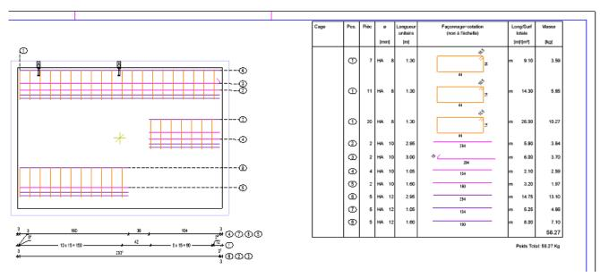
By using the tool "Assembly Group", it's possible to create an assembly of few reinforcement as a group.
