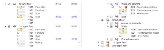
2 Select the Add to View tool and press CTRL+A twice to add all model data to all the sections.
