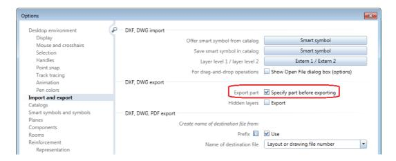
Basically, the elements displayed on screen should be the elements you want to transfer. In the **Transfer mode** area of the configuration settings, specify that the **Currently visible data** is to be transferred as 2D elements.
