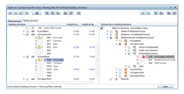
Note: This approach ensures that only the drawing files 900, 903 and 1000 are selected for the model data of the beam.
