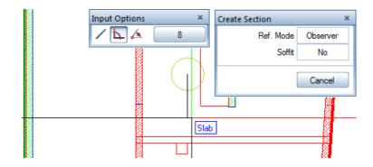
5 *From point - To point*: define the two diagonal points of the first clipping area in plan so that the entire downstand beam is included in the section. Press ESC to finish entering the polyline.
