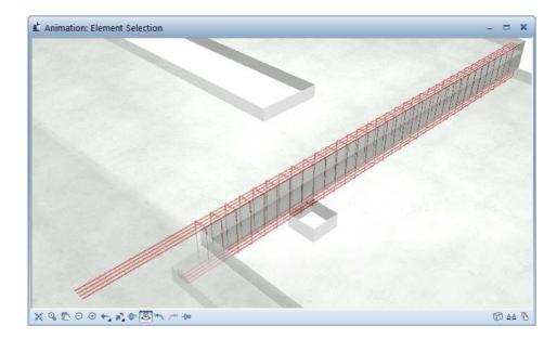
Note: The Concrete\_reinforced.surf surface (transparency: 50%) has been assigned to the concrete components so that the reinforcement is displayed in the animation of the reinforcement drawing. Alternatively, change the transparency setting of the Concrete.surf surface and save it as a new surface. However, this change applies to all the concrete components in the entire project.
