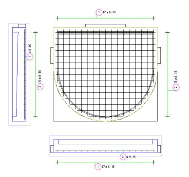
11 For layout output, all you need to do is hide the layer AR\_3D of the auxiliary box. This produces the desired reinforcement drawing.
