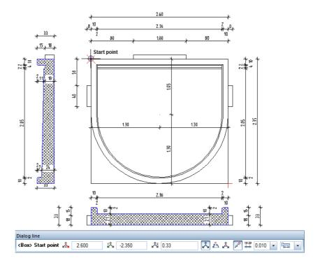
5 Change the reference mode to Folded and define the viewing direction by clicking to the right of the circle displayed on screen.
