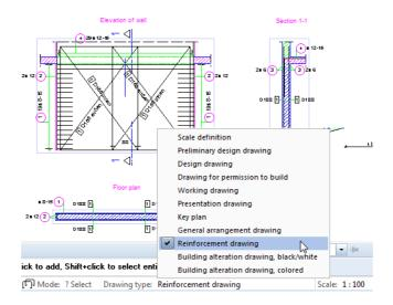
The on-screen display changes in accordance with the Reinforcement drawing plot set.
