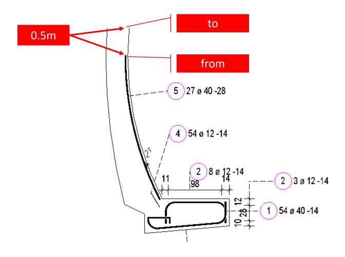
5. Is there any way to unfold a curved model or to correlate it with an orthogonal geometry? We want the following result, in which appears the unfolding of a tunnel, reinforced either with meshes, or with group of rebar's.
