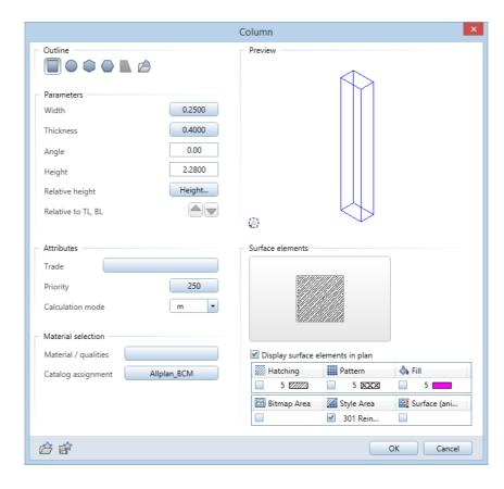
3 Set the parameters in the Column dialog box as shown above:
