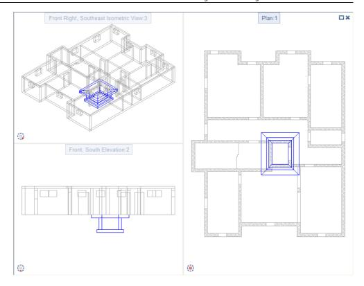
This elevator shaft and the floor plan of the basement will serve as the basis for exercise 4 that shows you how to create sections using the tools in the Associative Views module and apply reinforcement using the tools in the Bar Reinforcement module. Printing layouts is covered in exercise 9.
