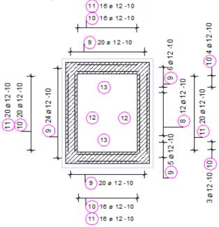
Now you have reinforced the elevator shaft with the exception of the horizontal corner reinforcement, which will be created using FF components. Finally, you will define the clipping area of the shaft walls.
