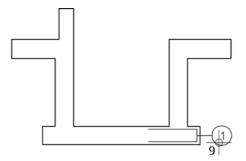
10 This defines the bending shape. If you want, you can continue and immediately place the open stirrup you just created. However, you can also press ESC and place the mark later using the Place Bar Shape or Special Placements tool. In this exercise you will place it now.
