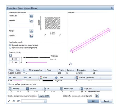
2 Set the parameters for the beam as shown above:
