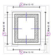
Floor plan of shaft walls t=30cm
