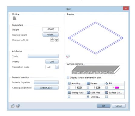
4 Click Height... and enter the height of the slab as absolute values. The unfinished floor of the ground floor = top level of the slab above the basement = -0.11. As the slab is 20 cm thick, the bottom level = -0.31.
