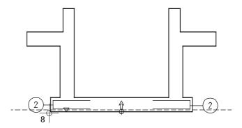
The dashed line indicates the current layer depth of the reinforcement. The concrete cover is taken into account. The elevation symbol shows the layer depth of the definition point entered. The direction of the positive bar segments and the placing direction of the bar are indicated by the arrow.
