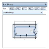
3 In the parameter area of the palette, set the diameter to 12 mm and clear the Same concrete covers check box, as these bars are in the second layer. Change the values for Concrete cover 1 and 3 to 0.055 each and the value for Concrete cover 2 to 0.04.
