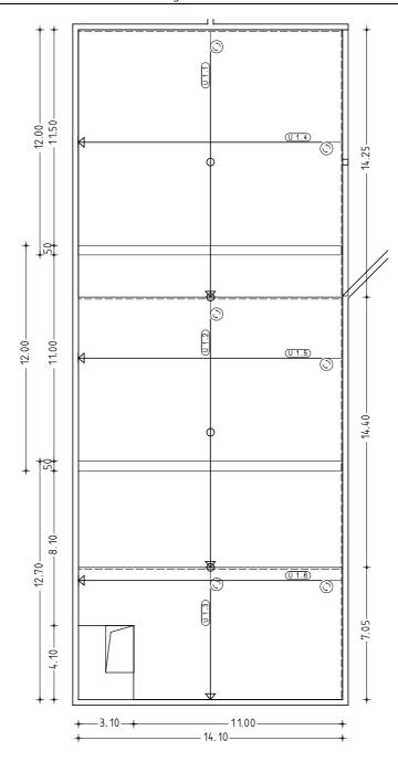
Before you can create the reinforcement for the carpets, you need to distribute the individual carpets in the placing drawing onto different drawing files. You will use carpet B1.1 as an example.
