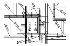
Start by placing open stirrups around the elevator shaft.
