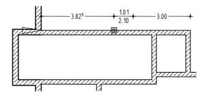
4 If the reference point is not displayed on the inside corner at top left, click on the corner to move it there and enter 3.825 m for the offset in the dialog line.
