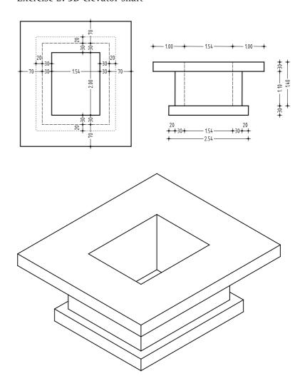
You will draw an elevator shaft for the basement created in exercise 1 using the tools in the 3D Modeling module. As an alternative, you will use the tools in the Basic: Walls, Openings, Components module.
