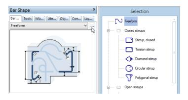
3 In the parameter area of the palette, se the diameter to 12 mm, enter 0.04 for the concrete cover and clear the Hook at start and Hook at end check boxes.
