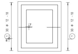
As an alternative, you will now use a predefined, expanding bending shape to create the edge reinforcement in the transverse direction. Finally, you will place the bending shape automatically.
