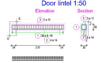
Next, you will alter the spacing in the middle of the beam using direct object modification. Finally, you will change the diameter of the bottom longitudinal reinforcement using the properties palette.
