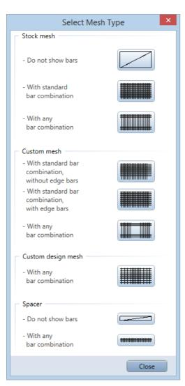
Stock meshes without a single bar representation; only the length, width and overlap are variable.
