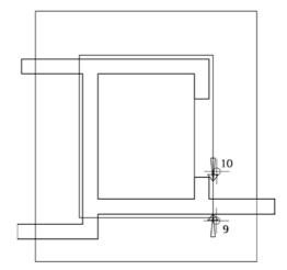
The placing region is highlighted in the floor plan of the shaft walls, and the placement is displayed in the floor plan of the floor slab. As the starter bars for the wall are not within the clipping area of the shaft walls, all the bars are displayed, regardless of the selected display mode.
