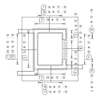
The floor plan of the floor slab also contains marks 9 and 10. You will now hide the wall reinforcement in this area.
