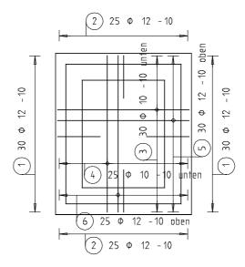
Instead of creating the top layer from scratch, you can copy and mirror the bottom reinforcement.
