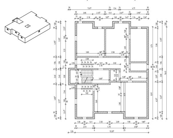
You will draw a basement in 3D using the tools in the Basic: Walls, Openings, Components module and in 2D using the tools in the Draft module.
