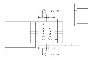
The longitudinal reinforcement is still missing.
