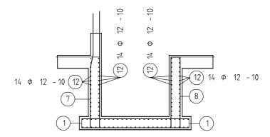
13 Now use the same procedure to create horizontal reinforcement for the transverse side. To enter the bending shape, select Expand to adapt to edges in the input options. Define a new placing line in the area of the shaft wall in section B-B. The start point of this new placing line is at the top and the end point at the bottom. Finally, hide the transverse reinforcement in the floor plan of the floor slab.
