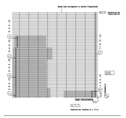
Reinforce carpet B1.4 yourself. The approach is the same as with carpet B1.1. The start point of carpet B1.4 is the bottom left corner of the carpet polygon. The additional reinforcement is spaced at the following intervals (reference point at top or bottom right):
