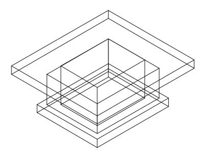
To finish, you will assign a surface element to the volume model. This surface element will be used later when you create associative sections. After this, you will move the volume model so that it is congruent with the 3D floor plan created in exercise 1. In addition, check that the top of the elevator shaft and the bottom of the basement walls are flush.
