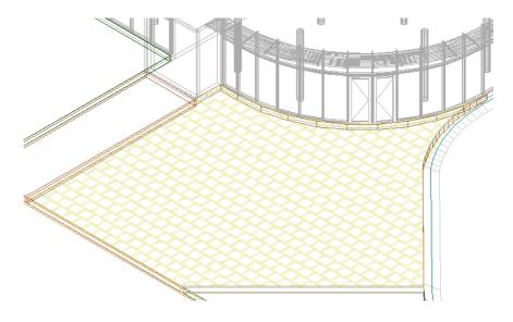
17 Delete the slab below the panels placed. Check the result in animation.
