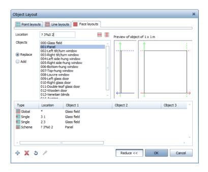
Each geometric element of the facade (point, line, face) has a location that is defined by the subdivision.
