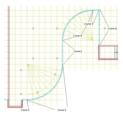
4 Click to open a new tab. Define the following settings for the first section of the facade (curve 1 = location 1), which consists of a straight line:
