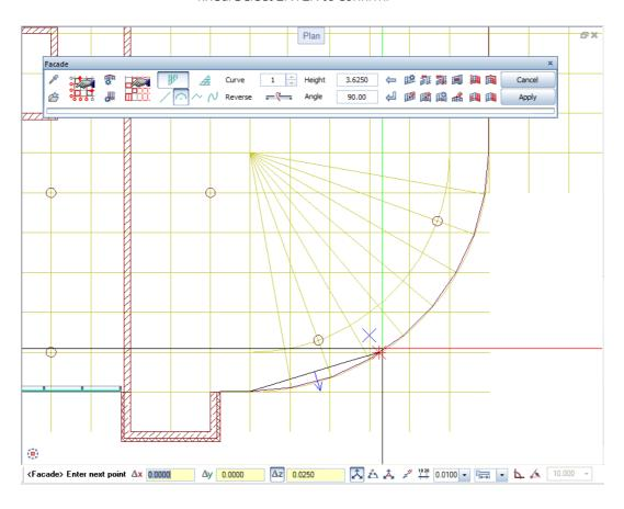
18 Point to the end of the arc. Here, too, the offset for  $\Delta z dz = 0.025$  remains fixed. Select ENTER to confirm.
