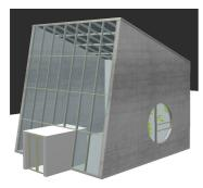
You can insert windows simply by clicking defined points, regardless of the shape of the opening. Thus, you can create window surfaces of circular, polygonal, and planar shape. There is no limit to creativity! Inserting a window only takes a few mouse clicks. You do not need any complex drafts. Just enter the parameters; Allplan automatically creates the window. You can use all the favorites to design the windows.
