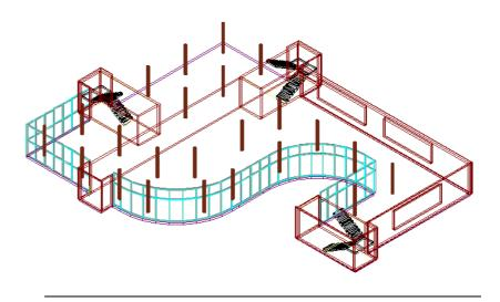
Finally, use the Modify tool to change the height of the facade section (curve 3) to 3.25 m. This is the section with the skyway on the upper floor.
