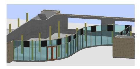
Note: The settings you define with Assign object apply even when you select a different Facade favorite. Therefore, reset these settings when you have finished assigning panels to the facade. Otherwise, these settings will affect other facades, such as the one described in Step 7: placements (on page 101).
