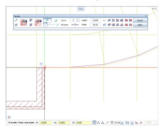
14 Point to the end of the straight line and enter  $\Delta z = 0.025$  in the dialog line.
