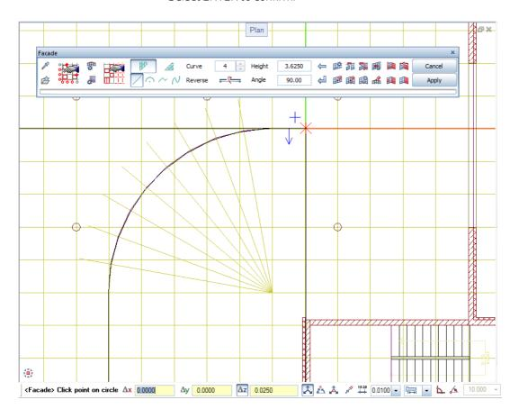
29 Point to the last point of the new facade. To correctly join the facade with the wall and floor, enter  $\Delta y dy = 0.025$  m in the dialog line;  $\Delta z dz = 0.025$ .
