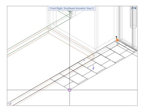
13 Zoom in on the required areas to place the panels along the corners of the slab.
